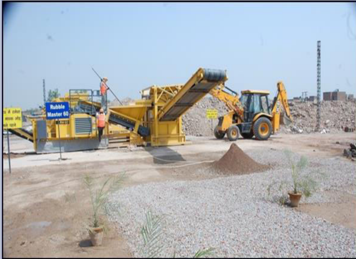
Crushing of C&D waste – dry process
